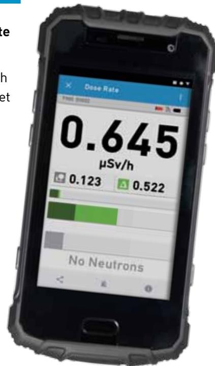
Target-Android-App on a mobile phone connected via Bluetooth to the F900.
