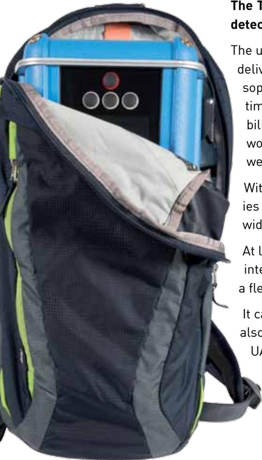
**The Target F900 is a radio-nuclide identifier with a large single NaI<sup>L</sup>™ (NaI:TI, <sup>6</sup>Li) detector (2" x 4" x 8") packed into a rugged watertight housing.**
