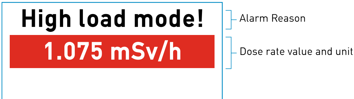
The high load screen still displays a valid dose rate.
